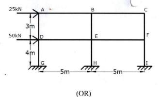
Analyse the frame shown in figure by Portal method. Draw column bending moment diagram and beam bending moment diagram.
