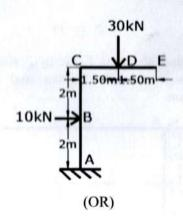
5. The load system shown in figure crosses a plate girder bridge of span 30 m from left to right. Determine the maximum bending moment and shear force at section 8 m from left support. Also find the absolute maximum bending moment.
