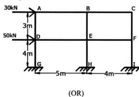
Analyse the frame shown in figure by Cantilever method.
